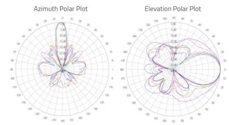
Start Frequency: 2300 MHz Stop Frequency: 2700 MHz
