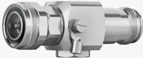
The Telegärtner Surge Protector (SKU: ACC-TG-00008) is a high-performance RF surge protector designed for 4.3-10 Male to 4.3-10 Female connections, supporting frequencies up to 3.8 GHz. This makes it ideal for 5G networks and advanced communication systems. It utilises a Gas Discharge Tube (GDT) to protect sensitive electronic equipment from high voltage surges, with a discharge capacity of up to 40 kA (8/20 impulse).
