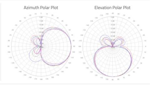
Start Frequency: 1710 MHz Stop Frequency: 2700 MHz
