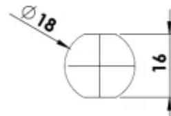
Max. mounting thickness 12mm
