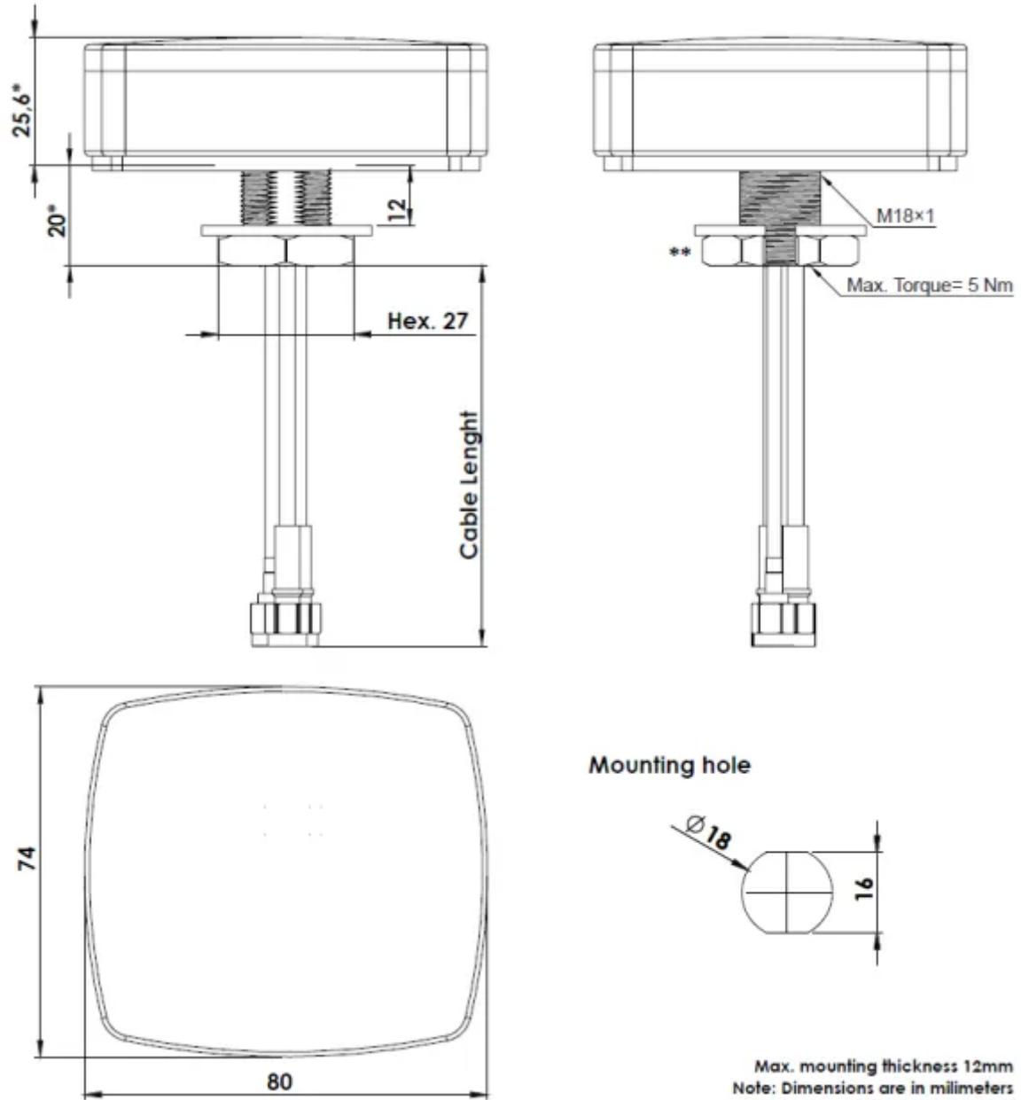
Max. mounting thickness 12mm
