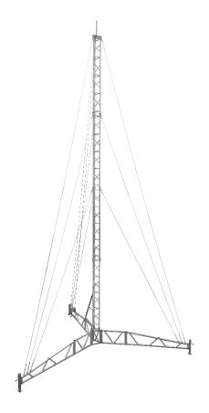
APAC's AL340 aluminium lattice modules feature three upright columns made from 50x4 CHS with 32x3 CHS lattice welded in between by certified boom welders, providing incredible strength while retaining a lightweight design that can support your technician to climb the full 14 metres. The three hinge feet are machined from 76.2 mm solid billet 6005 T5 aluminium, providing unmatched strength with precision machining ensuring perfectly distributed load across bolts and galvanised receptacle.
