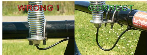
Route the RG58 low loss stranded cable carefully. Avoid high heat areas such as hot components within an engine bay. Ensure that the cable is not stretched excessively and there are no sharp kinks. Use cable ties, but do not pull so tight as to crush the cable. A damaged feeder cable is a cause of high VSWR and reduced performance.
