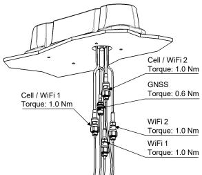
Connect the cables. Apply the indicated torque according to the connector.
