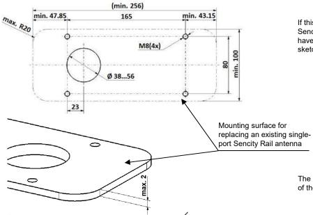
If this antenna will replace an existing single-port Sencity Rail antenna, the mounting surface must have the minimum dimensions as shown in the sketch.
