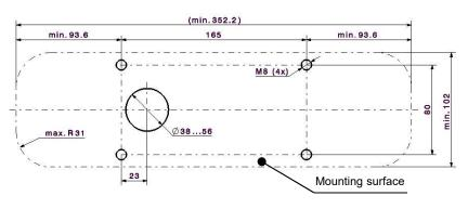
Find a suitable mounting surface and drill the mounting holes according to the sketch.
