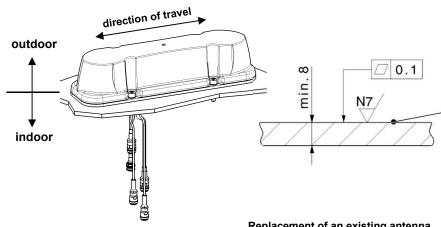
The mounting surface shall be planar and stable. The material of the mounting surface shall be steel or aluminium.
