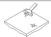
Clear the area where the antenna is mounted from paint, corrosion, anodized layer, dust, cutting chip, oil and fat.
