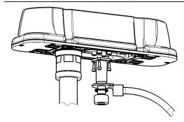
When mounting the antenna onto a bracket, the cable entry has to be protected against environmental impact. If the mounting surface doesn't fulfill the requirements mentioned above, the antenna has to be grounded using a separate grounding cable.
