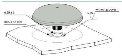
Drill the mounting hole (ø 29 ± 1 mm).
