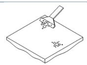
Clear the area where the antenna is mounted from paint, corrosion, anodized layer, dust, cutting chip, burrs, oil and grease.
